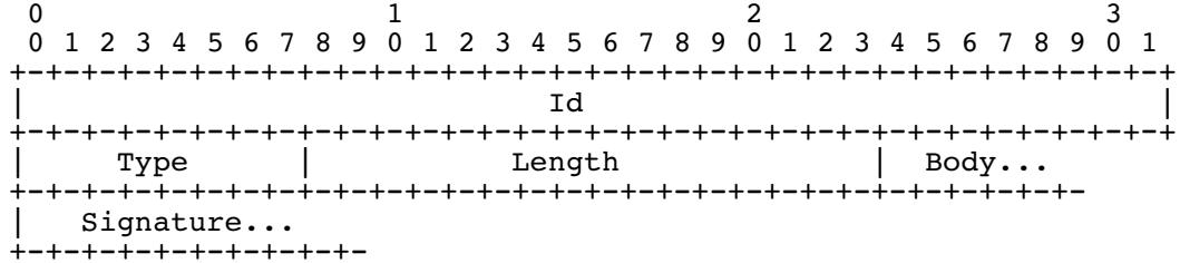
The field *Type* indicates the type of the message; values 0 to 127 indicate requests, values 128 to 255 indicate replies. The field *Id* is arbitrary in requests, and is copied from the request to the reply. The field *Length* indicates the length of the field *Body*.
