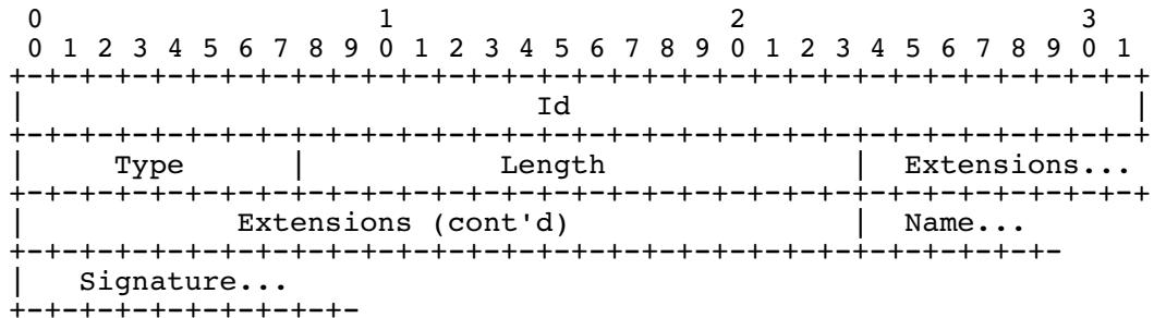
The field *Extensions* is a 32-bit bitmap of supported protocol extensions (optional features), see 4.2. The field *Name* contains the name of the sending peer.
